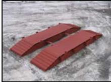
Each pad is separated by the same distance that exists in between the machinery's tracks or wheels. This type of installation requires (2) tie down spacer bars to secure both sections in a safe position. This is the most popular type of installation.
